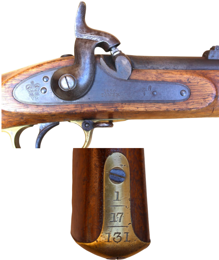
A .577" PATTERN 1856, 2 BAND PERCUSSION VOLUNTEER RIFLE BY GEORGE DAW, CIRCA 1860, with 33" barrel rifled with 3 grooves, fitted with a bayonet lug at muzzle and ladder rear sight, engraved at breech "GEORGE H. DAW, 57 THREADNEEDLE ST. LONDON", borderline engraved lock marked G. DAW to centre, iron mounted full walnut stock with chequered wrist and forend in typical G. Daw style. A typical Pattern 1856 volunteer rifle with distinctive Daw style chequering, in very good condition with v. good stock quite sharp overall, barrel to a fading blue / grey patina, very good bore with sharp rifling. £795
