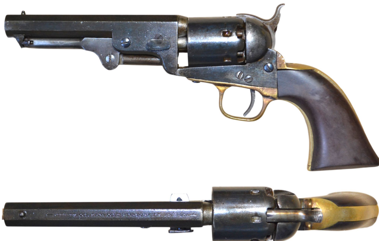
A 54 BORE WEBLEY BENTLEY SELF COCKING PERCUSSION REVOLVER, with 5 ½" octagonal Birmingham proofed smoothbored barrel, the top strap engraved 'PATENT LONDON', fitted with Kerr type loading lever, five shot cylinder, two-piece barrel and frame, two piece chequered walnut grips, In very good condition professionally reblued, the left grip with some bruising, Bentley patent nose catch removed. (38/54) £495
